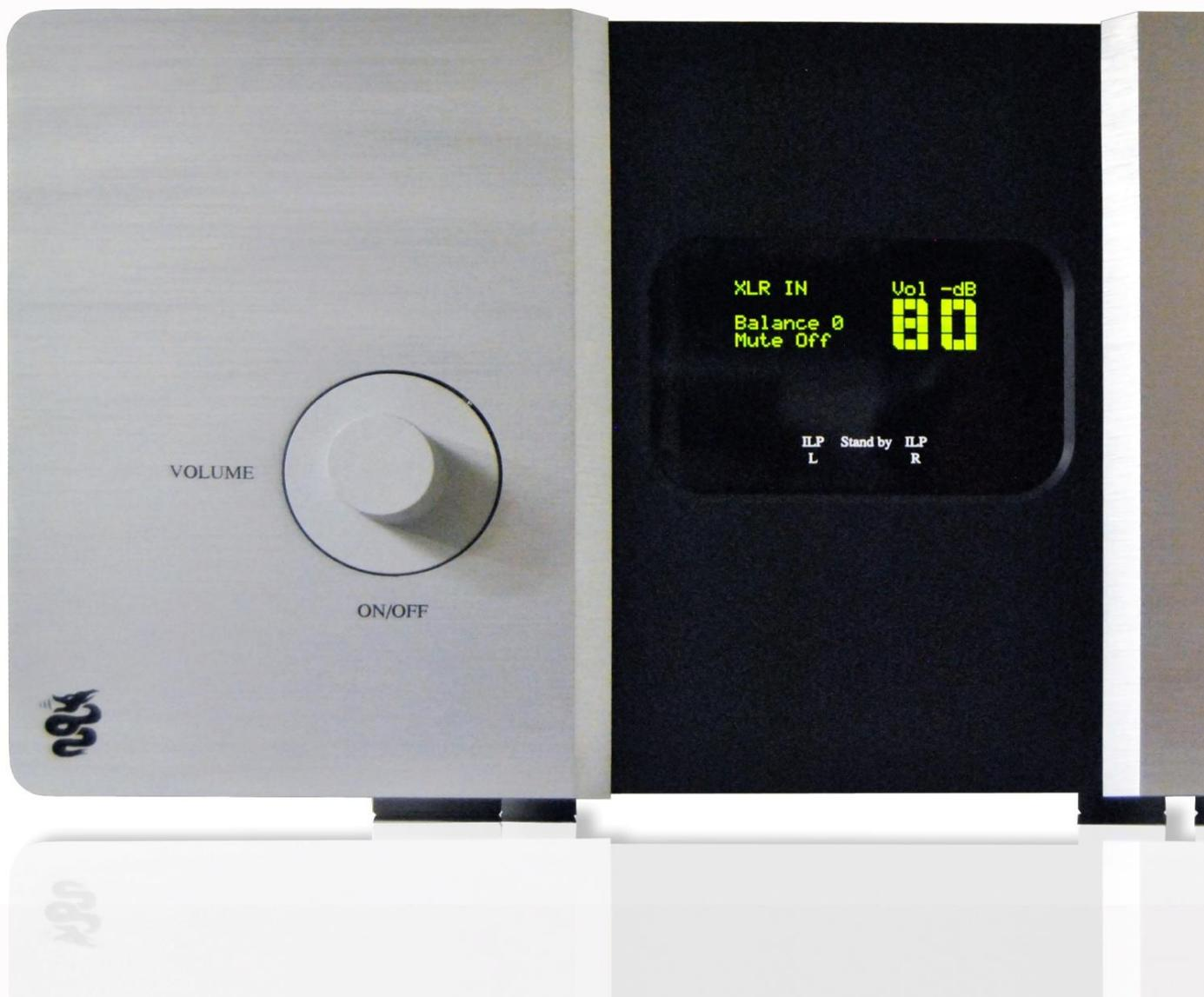
*Power and unprecedented headroom - massive steel chassis no damping - class A - dual mono configuration - Burr Brown digital potentiometer PGA2310 - OLED display for optimal viewing angle - protection system owner - double sided PCB 70 microns - stage input equipped with components from "instruments" for outstanding sonic transparency*
