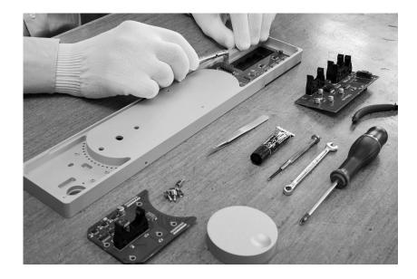
The products manufactured by B.audio are handmade in the company's workshops in Mutzig, near Strasbourg. The assembly of the electronic boards as well as the crafting of the housing components are carried out locally by partner companies. Each element is tested both electronically and acoustically to validate its performance at the end of assembly.
